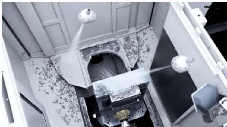
Figure 24: "AI Chip Removal" application from DMG MORI for the removal of chips by Artificial Vision 146
