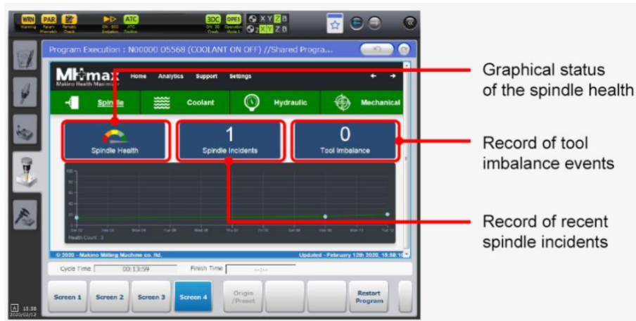
Figure 22: “MHmax” Software of Makino to determine the spindle status 136
