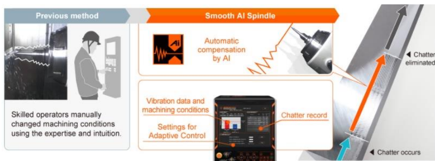
Figure 23: “Smooth AI Spindle” system of Mazak 138
