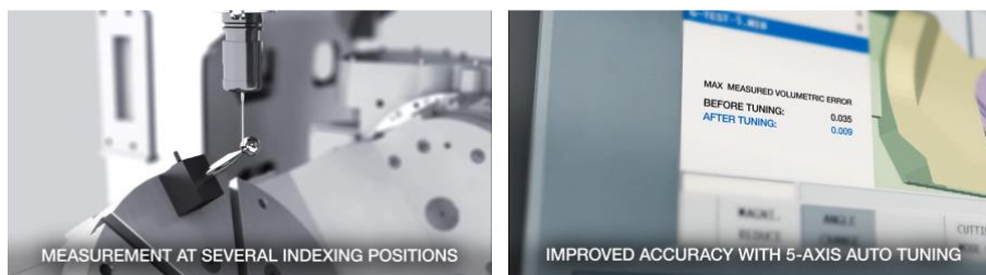
Figure 12: 5-Axis Auto Tuning of Okuma 86
