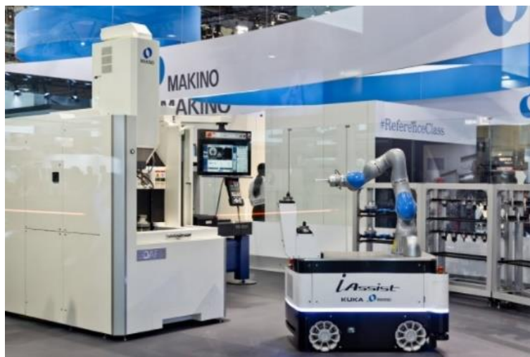
Figure 27: Robot i-Assist by Artificial Vision of Makinol
