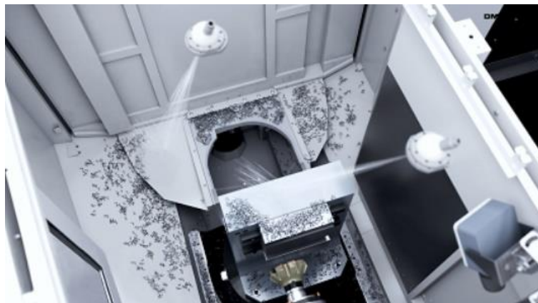
Figure 24: "AI Chip Removal" application from DMG MORI for the removal of chips by Artificial Vision 146
